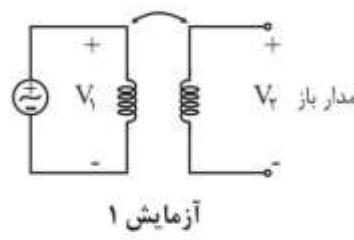
$$\begin{aligned} k &= \left| \frac{V_2}{V_1} \right| \times \left| \frac{V'_1}{V'_2} \right| & (1) \\ k &= \sqrt{\left| \frac{V_2}{V_1} \right| \times \left| \frac{V'_1}{V'_2} \right|} & (2) \\ k &= \left( \left| \frac{V_2}{V_1} \right| \times \left| \frac{V'_1}{V'_2} \right| \right)^{\frac{1}{2}} & (3) \\ k &= \left| \frac{V_2}{V_1} \right| \times \left| \frac{V'_2}{V'_1} \right| & (4) \end{aligned}$$
